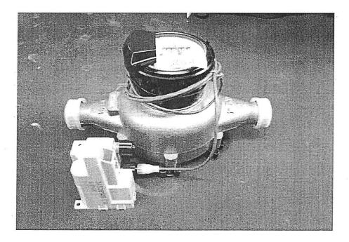
Actual picture of an Itron 100W Water ERT Module from the Water Utility inventory attached to a one inch water meter. The Itron module transmits the meter reading wirelessly to the meter reader. This eliminates the meter reader from entering residential homes, commercial business's and underground meter pits for getting meter readings for billing purposes.
